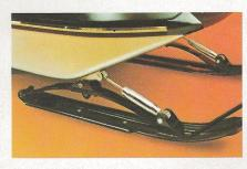
A super smooth ride and positive steering is assured by Boa-Ski's combination leaf spring and shock dual front suspension system on SS and Mark II models. Mark I and Mark 230 models feature cushion-flex spring front suspensions, perfectly suited for lighter duty snowmobiles.
