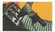
SS performance riders will appreciate the added control provided by this Kelsey-Hays hydraulic disc brake system. A gentle squeeze is all it takes to bring this booming super-sled to a smooth, safe, controlled stop. All other Boa-Ski models feature an easily-actuated mechanical disc brake, engineered for sure stopping at all speeds. All Boa-Ski models come with thumb throttles for easy acceleration and smooth, fatigue-free cruising.
